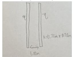
a. Because I am given the distance and the area for parallel plates, I will use:  $C=Ae_0/d$ .  $e_0$  is always 8.85e<sup>-12</sup> C<sup>2</sup>/(N\*m<sup>2</sup>)
