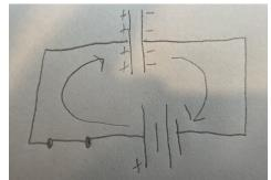
4. Capacitors in parallel: For capacitors in parallel, Vbattery = V1 = V2
