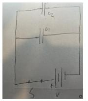
5. Capacitors in Series: For capacitors in series, Qbattery = Q1 = Q2
